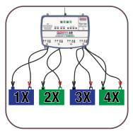
CAN CHARGE FOUR 12V & 12.8V BATTERIES INDEPENDENTLY
